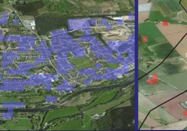
Ground uplift of 2.5 - 3 cm over a period of 1 year was detected for this sub-urban area. Ground subsidence of 2 cm over a period of 1 year was detected near natural gas pipeline site
