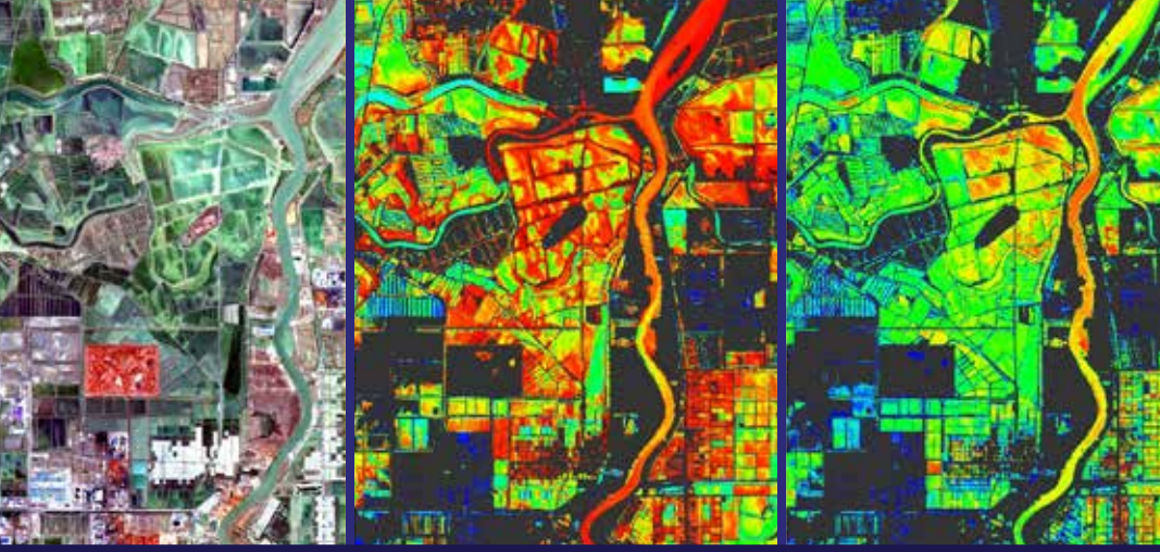
Water Quality of Aquafarms in Bohai Bay, China - (L) True Color (M) TSM (R) CHL
